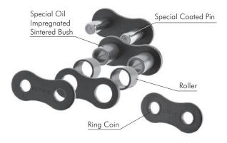
Fig. 23 Basic Construction
