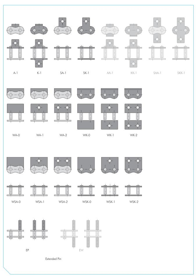
Fig. 3 Overview Single Pitch Attachment Types
